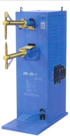
The DN sery point welder is a foot drivepoint welder. It is mainly use to point weld low carbon steel plates, and weld two plate materials or line materials if you grasp good welding technics, you can point-weld some piece of nonferrous metal and alloy.
